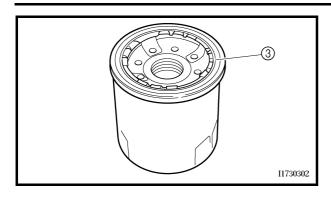
• Lubricate the O-ring ③ of the new oil filter cartridge with a thin coat of engine oil.
