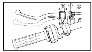
• Turn the brake lever cable adjusting nut (drum) ③ clockwise until the gap ④ is within the specified limits.
