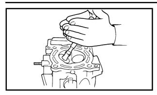
• Apply a fine lapping compound to the valve face and repeat the above steps.
